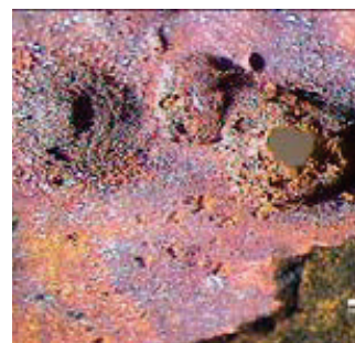
Beautiful but undesirable. Electron-microscope image of copper corrosion products.
